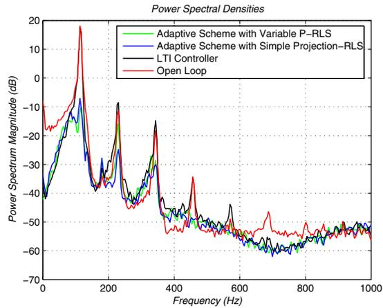
Fig. 12. PSDs of the Outputs (8000 Samples).
