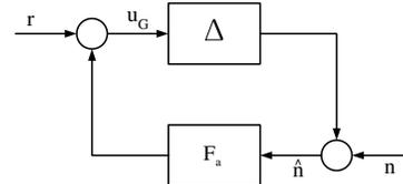
Fig. 3.  $\Delta$  and  $F_a$  in Typical Feedback Connection.
