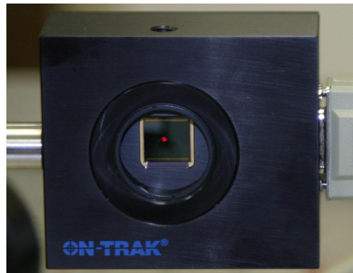
Figure 4. On-Trak Optical Position Sensor. Axis 1: horizontal; Axis 2: vertical. Control objective: maintain red laser spot at center of sensor.
